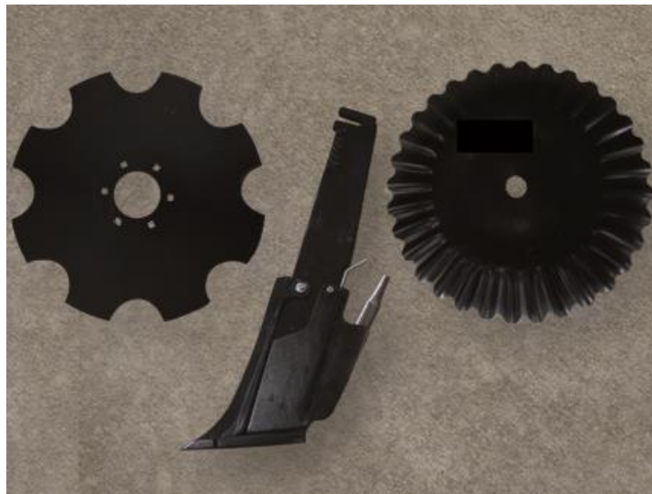
Disks (left), shanks (middle), and coulters (right) are commonly found on tillage equipment. Credit: Addison Dahmer
